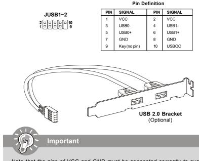
Note that the pins of VCC and GND must be connected correctly to avoid possible damage.
